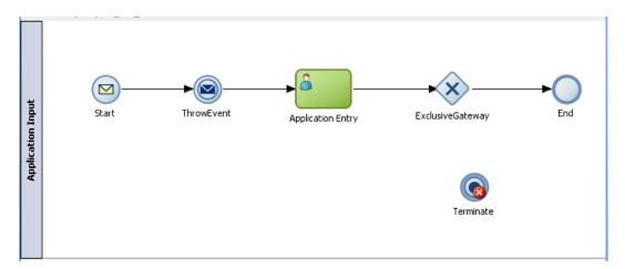
Right click on the **gateway** and select the **Add Conditional Sequence** flow, and connect the gateway to the **Terminate event**.
