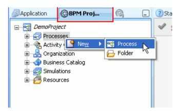
In the BPM Process wizard, select the Asynchronous Service pattern.
