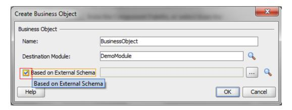
On click of Search Icon the following window appears, now click on the Icon at right most Corner to browse the location of the **xsd** that is to be loaded. For example **txn.xsd** in this project is loaded. After loading the **xsd**, it prompts for the copy of the **xsd** to the project. Click Ok. So that the **xsd** is copied to the project.
